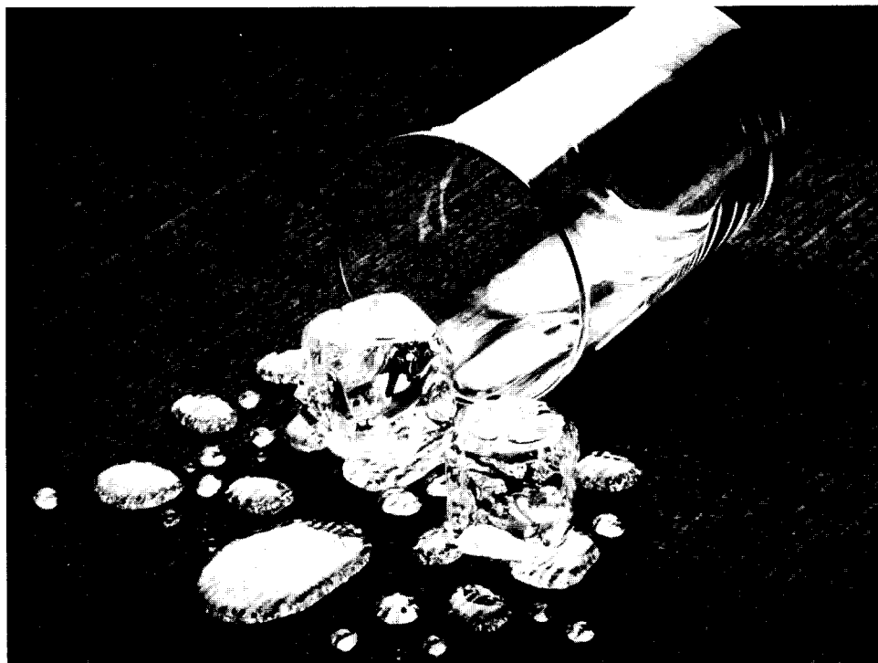
Fig. 11.6. Fluids resistance of fluorinated fabrics. (Photograph reproduced by permission of the Commercial Chemicals Division/3M, St. Paul, Minnesota, U.S.A.)
